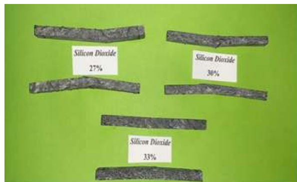
Figure 3: Deformation specimens after testing
